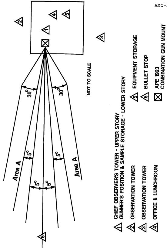
Figure 22-5. Typical small arms trace test range
